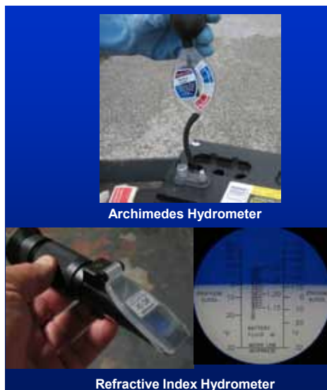
Figure 117. Hydrometers measure electrolyte specific gravity (SG).
