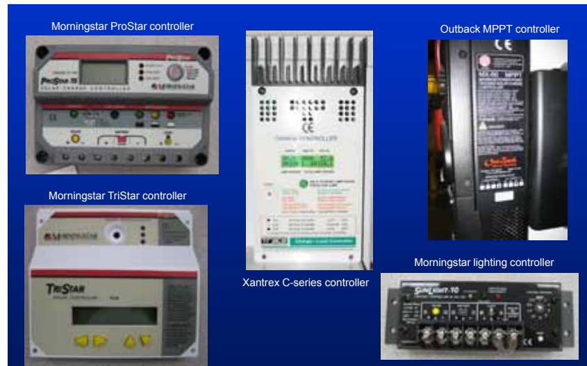
Figure 33. Charge controllers used in PV systems vary widely in their size, functions and features.
