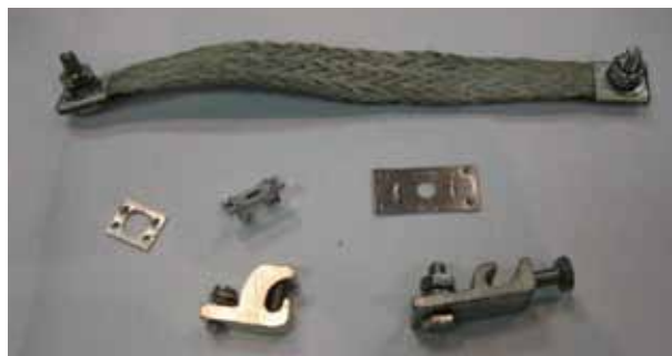
Figure 98. Special bonding jumpers, stainless-steel bonding washers and lay-in lugs may be used to electrically connect separate components or attach equipment grounding conductors.
