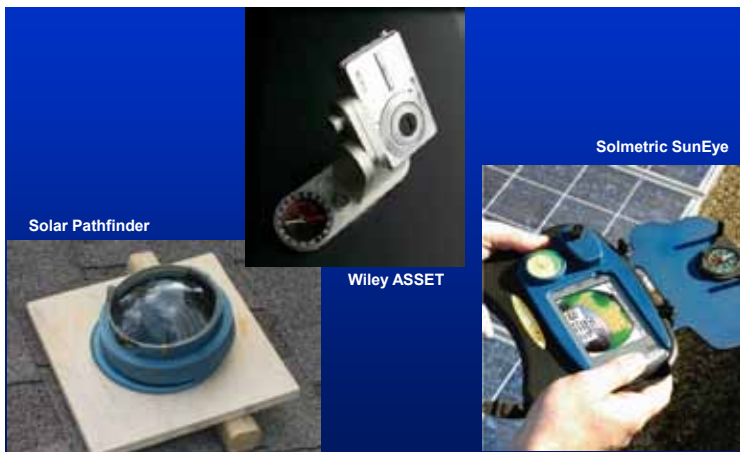
Figure 18. Various devices are used to determine the extent of shading for potential PV array locations.
