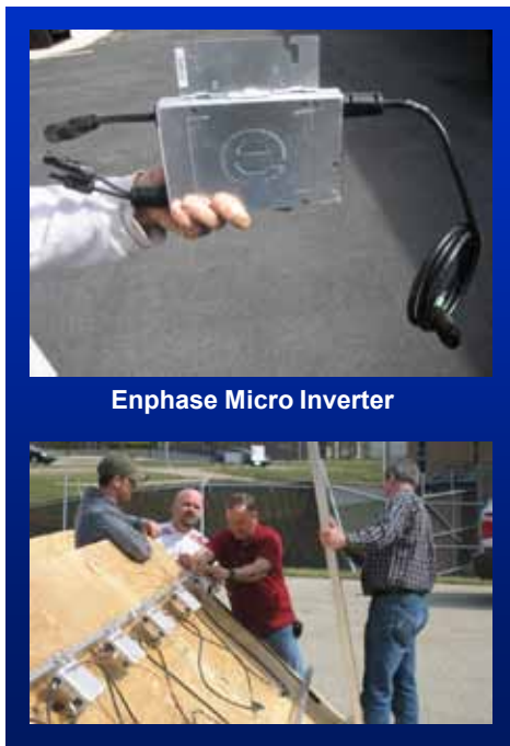
Figure 72. AC modules and micro inverters are small inverters installed integral to or adjacent to individual PV modules.
