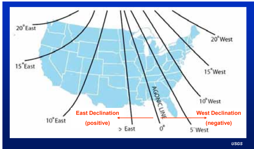
Figure 12. The western U.S. has positive (easterly) declination, and will cause a compass needle to point east of geographic north.
